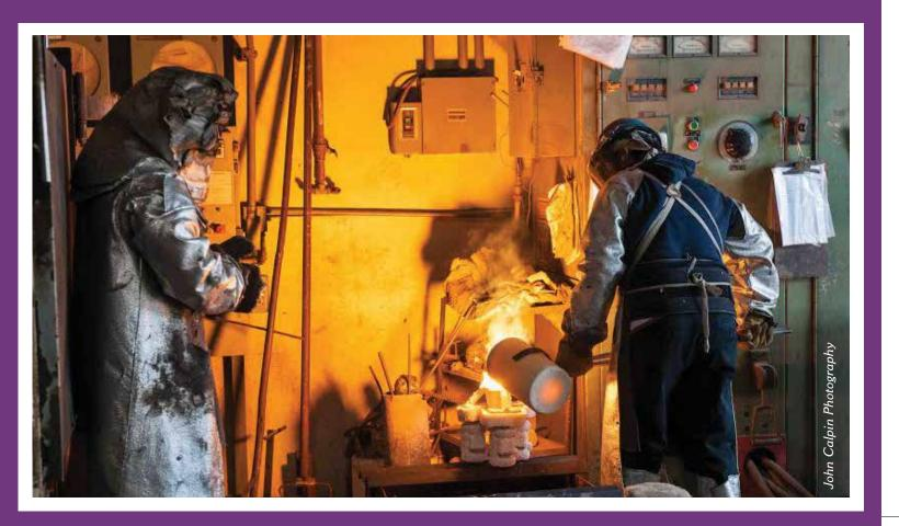
stand with the pouring funnel on top. Molten bronze heated to 2,200 degrees is poured into the funnel and travels down through the sprues into the cavities of the shell. As the bronze cools, the positive is created.
